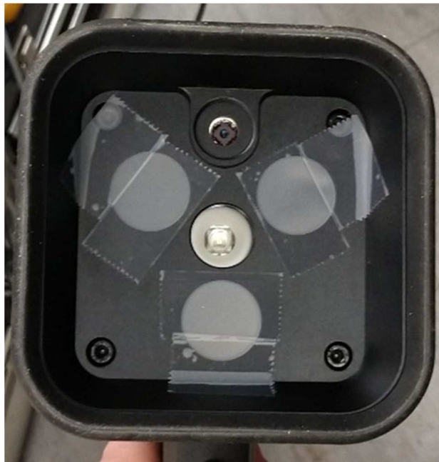
Figure 12. Camera with Three Taped up UV Lights
