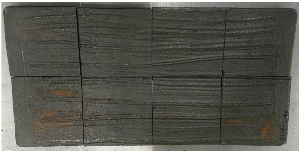
Figure 9. Sample Cut into Eight Pieces from Cope View
